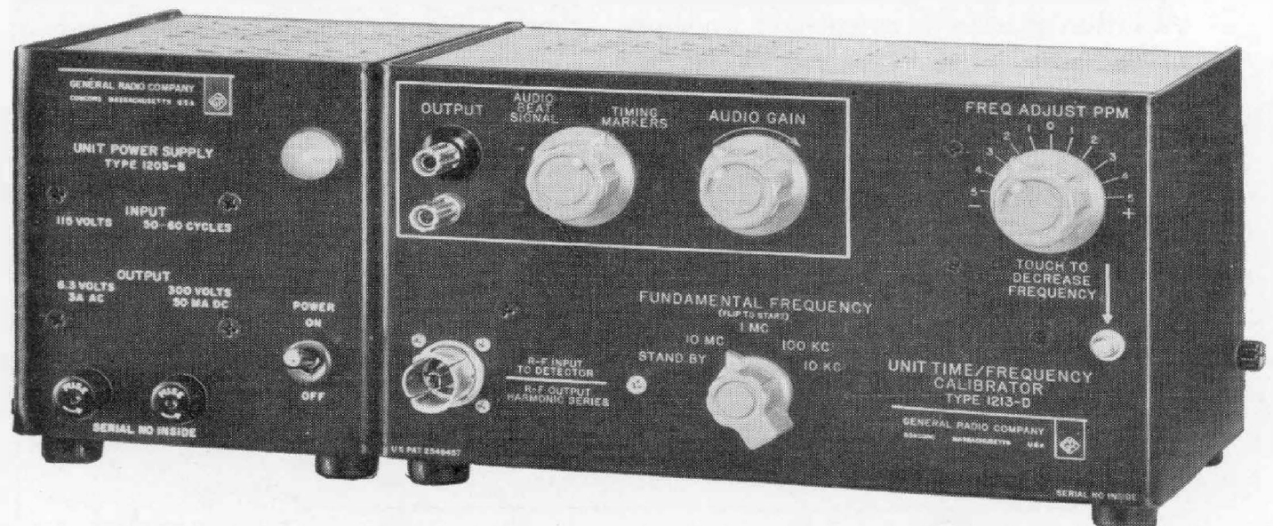
Figure 1. Panel view of the Type 1213-D Unit Time/Frequency Calibrator with Type 1203-B Unit Power Supply.
